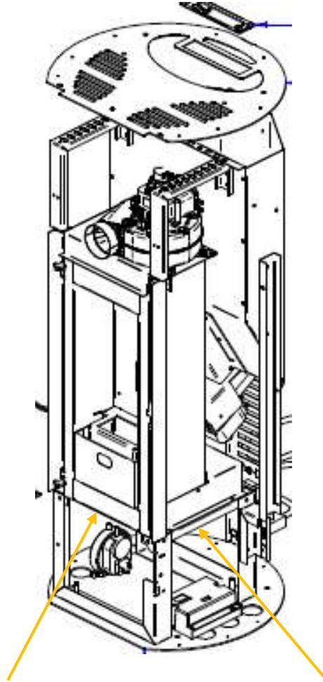
FOR THE CLEANING OF THE STOVE'S FURNACE IN THE FIRST SERIES, THE BOTTOM OF THE STOVE (WHERE THE FUME EXTRACTOR ENGINE IS FIXED) MUST BE DISASSEMBLED BY UNSCREWING THE VARIOUS SCREWS THAT ARE FIXING IT.
